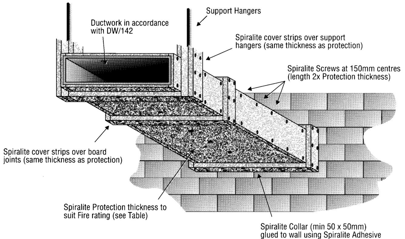
**NOTE:** 3mm stud welded pins to be fixed on soffit of ducting, 300mm from each edge and at 600mm centres. 38mm diameter non-return washers to be used to secure cladding on pins. Pins to be bent through 90°.
