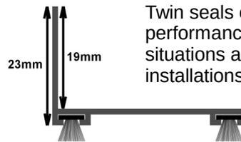
Twin seals offer superior sealing performance, particularly in under door situations and to sides of sliding door installations. DLB & DLF Seals come with slotted holder for simple installation or adjustment.
