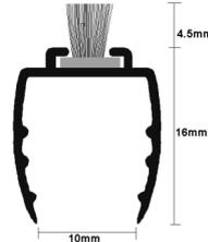
12mm Glass edge seal in clear PVC extrusion with black brush protruding 4.5mm out of holder.
