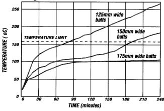
This graph was prepared from data recorded during a pilot furnace examination of the product conducted by the Commonwealth Experimental Building Station.
